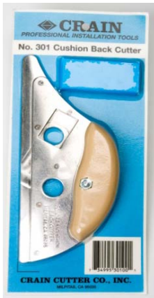
Cushion Back Cutter Part # 301 - $26.95 This tool is designed for tight weave gauges of rubber back carpet. It has a blade slot on both sides for cutting either side of the row, and the 30° blade angle prevents tearing. It has a stainless steel construction. Includes five blades.
